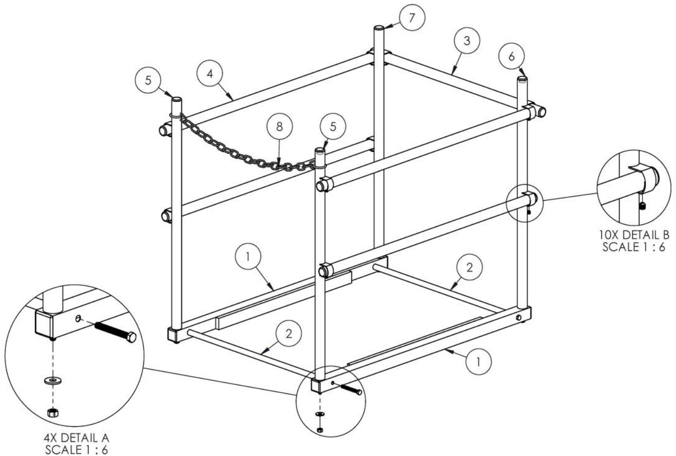
**General:** Safety railings are designed to mount on roof hatches to provide fall protection around the hatch when open. The following instructions are recommended general guidelines for installing compression type safety railings.
