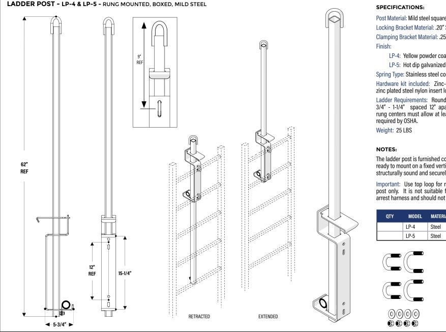
Post Material: Mild steel square tubing 1-1/2" x 1-1/2" x 1/8" Locking Bracket Material: .20" Steel Plate Clamping Bracket Material: .25" Steel Plate
