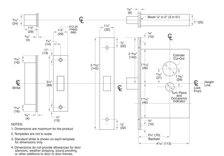
ANSI Standards: L400-Series locks meet all requirements for installations in doors and frames prepared in accordance with
