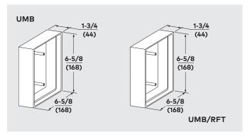
**UMB** — Black ABS universal replacement mounting box for WS-1 type switches.
