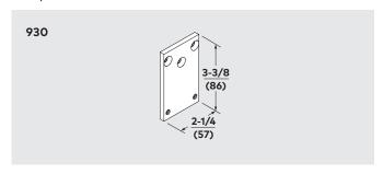
**930** — For mounting arm shoe in top jamb drop application when top door rail is less than 4-5/8" (2" minimum required).
