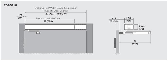
**NOTE:** Refer to the included bumper/stop to limit door travel to a maximum 110° to prevent possible damage to the ED900 arm. Where this is not practical, the ED900 J × Drop Mount with a surface door stop is recommended.
