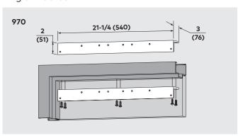
970 — For mounting ED900 J easily on deep reveal frame conditions or when frame face is less than 1-3/4".
