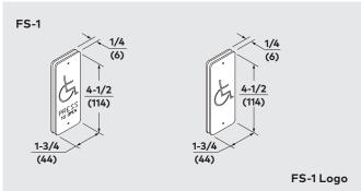
**FS-1** — 1-3/4" × 4-1/2" frame plate with a normally open switch. Satin stainless steel frame plate with blue engraving. Frame plate displays the accessibility symbol and "PRESS TO OPEN." Fits a minimum 1-3/4" × 4" frame section. Must be hard wired.
