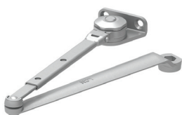
4040XP-3049 Hold-open arm Non-handed Mounts pull side or top jamb with shallow reveal, hold-open adjustable shoe 4040XP closer includes 4040XP-62PA shoe required for parallel arm mounting Optional
